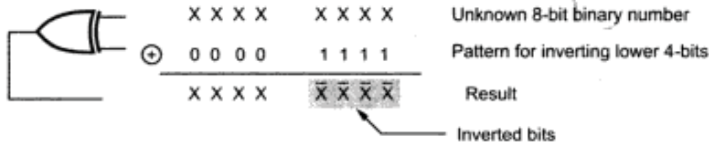
Fig. 3.16 Inversion of part of a number using XOR operation
