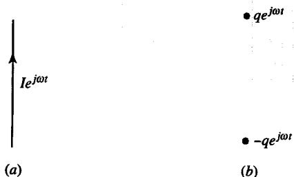
Figure 2-2 Ideal dipole models. (a) Uniform current model. (b) charge dipole model with I = j\omega q .
